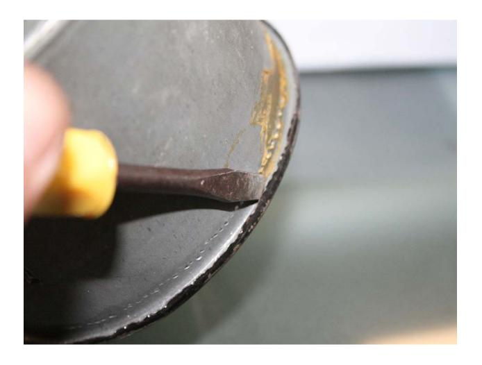
3. Now take the flat head screwdriver and place it between the trim ring and speedo housing and gently begin to separate the 2 pieces. Work your way around the speedo until the trim ring is loose enough to remove by hand.
