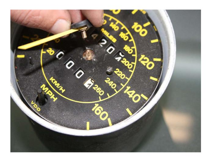
6. Now remove the 2 small black screws that hold on the faceplate. Once the screws are removed lift the faceplate out of the way.
