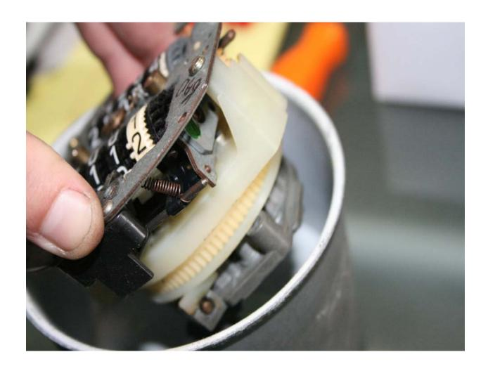
9. Now turn the speedo in your hand until you get the the red odometer gear. To remove this gear use a flat head screw driver to pry the gear up the shaft until it is removed.
