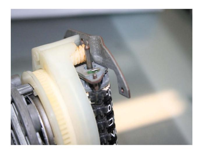
10. Now before you can put the new gear back on the shaft you must wedge a flat head screwdriver on the other side of the odometer gear shaft to prevent it from sliding while you are putting the new gear on. The gear is a very tight fit and it will require some force to push it on the shaft. You can use a screwdriver to push the new gear on the shaft but only apply pressure to the collar of the gear do not apply pressure to the edges or you may damage the gear.
