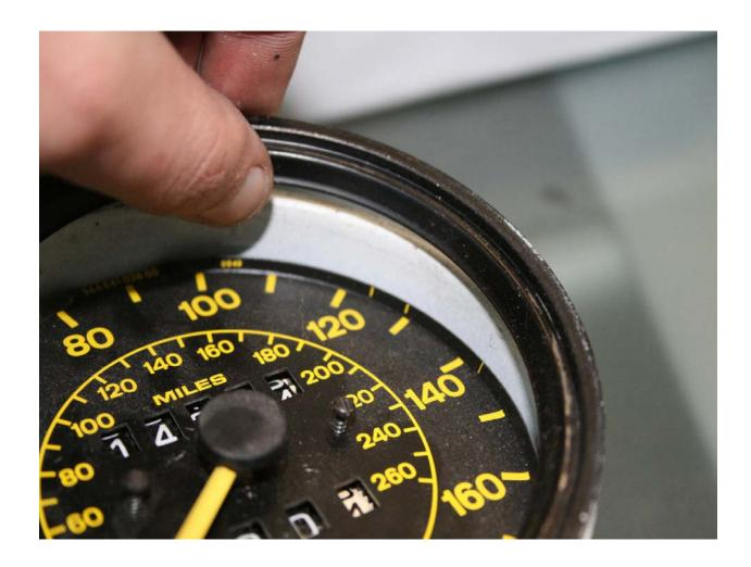
5. Now to remove the needle lift straight up on the needle with your fingers as your are turning it all the way to the right towards the odometer reset button. It is important that you lift straight up on the needle do not jerk it or lift on a angle or you may break the shaft that the needle sits on. You may need to move the needle all the way forward and all the way back a few times before the needle comes off just continue to lift up while you are moving the needle in either direction.
